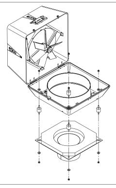
5 The fan assembly can now be fitted onto the steel chimney.
