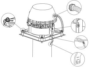
8 To avoid rainwater from entering the chimney fan the slots and holes must be sealed with silicone.
