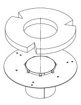
Fixate the flange to the chimney fan with the use of the vibration dampers supplied with the flange.
