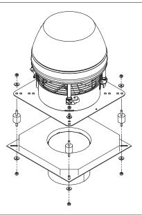
The fan assembly can now be fitted onto the steel chimney.
