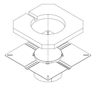
Fixate the flange to the chimney fan with the use of the vibration dampers supplied with the flange. The fan assembly can now be fitted onto the steel 5
