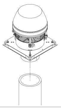
Use the safety wire to secure the fan to the chimney. Apply the supplied self-cutting screw in steel chimney. Then mount the wire through the designated hole in the base plate and into the wire lock.
