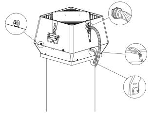
To avoid rainwater from entering the chimney fan the slots and holes must be sealed with silicone.
