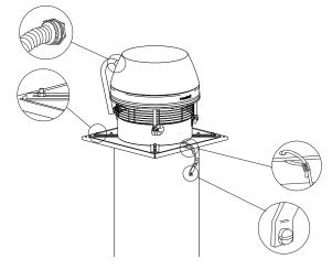
8 To avoid rainwater from entering the chimney fan the slots and holes must be sealed with silicone.
