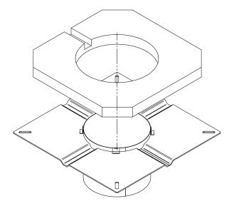
Fixate the flange to the chimney fan with the use of the vibration dampers supplied with the flange.
